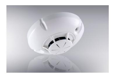
**FD8020** Rate of rise heat detector – The fire detector provides reliable early warning of a Fire condition upon reaching a rate of rise of the temperature or fixed temperature threshold in the protected premises. It is available in two versions (A2R or BR) depending on the temperature threshold in accordance with the European Standard EN54-5. The fire detector is suitable for premises with normal ambient temperature, without possible sudden changes.
