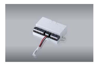
**FD7201S** Conventional line monitoring module – It is designated to connect conventional fire alarm line (with up to 32 fire detectors) as a part of the addressable fire alarm system IFS7000. The built-in short circuit isolators are available. **FD7201S** is power supplied via the power loop and up to 125 modules can be connected in each of the signal loops. It satisfies the requirements of the European Standard **EN54-17 & EN54-18**.
