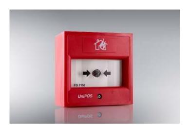
**FD7150** Manual Call Point – It is designated to release a signal for a Fire condition to the Fire Control Panel IFS7002 upon manual activation by breaking the glass on the place, signed with arrows. The light indication for activating the manual call point is provided by a red LED. There is possibility for testing by a special key. It satisfies the requirements if the European Standard EN54-11 for a type A manual call point and EN54-17.
