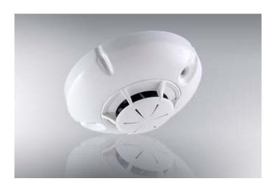
**FD7110** Fixed temperature heat detector – The fire detector provides reliable early warning of a Fire condition upon ambient temperature reaching a fixed temperature threshold. The temperature class (A1S, A2S or BS) is in compliance with the European Standard EN 54-5 and is programmable by Fire Control Panel IFS7002. The fire detector is suitable for premises with normal and high ambient temperature, with possible sudden changes.
