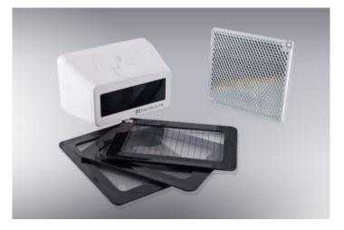
The DOP-40 beam smoke detector is designed for detection of smoke, nascent at the beginning stage of fire. It is especially suitable for protection of rooms, in which appearing of smoke, in the first phase of fire origin, is expected. This type of fire detector is, also, recommended for protection of places, where, due to large protected area, would be necessary to use of large number of point smoke detectors.
