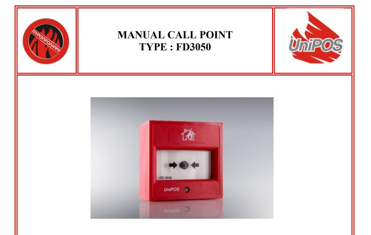
**FD3050** Manual Call Point – It is designed to release a signal for a Fire condition to the Fire Control Panel upon manual activation by breaking the glass on the place, signed with arrows. The light indication for activating the manual call point is provided by a red LED. There is a possibility for testing by a special key.
