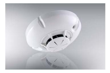
**FD7120** Rate of rise heat detector – The fire detector provides reliable early warning of a Fire condition upon reaching a rate of rise of the temperature or fixed temperature threshold in the protected premises. The temperature class (A1R, A2R or BR) is in compliance with the European Standard EN54-5 and is programmable by Fire Control Panel IFS7002. The fire detector is suitable for premises with normal ambient temperature, without possible sudden changes.
